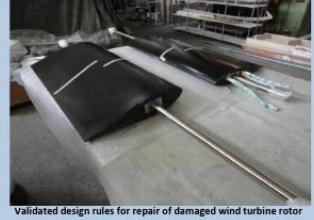
Validated design rules for repair of damaged wind turbine rotor blades (REWIND) Wing models for wind tunnel tests at EMIT (NTUA)
