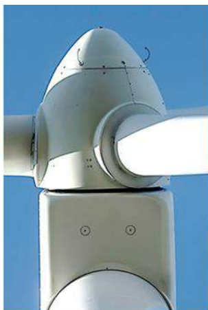
Mounting: Three 1D sonic sensors mounted axially between blades at positions where wind speed is close to free wind speed
